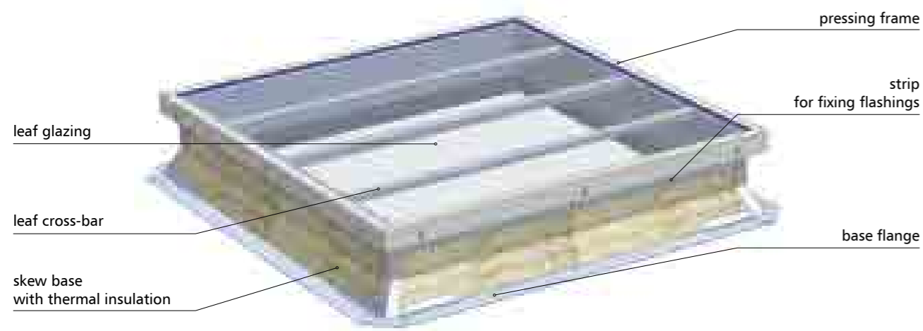
Fig.16 mcr PROLIGHT NG-A fixed skylight design
