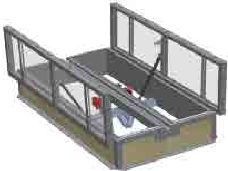
Fig.70 Design of mcr PROLIGHT DVP smoke vent equipped in mechanic control system
