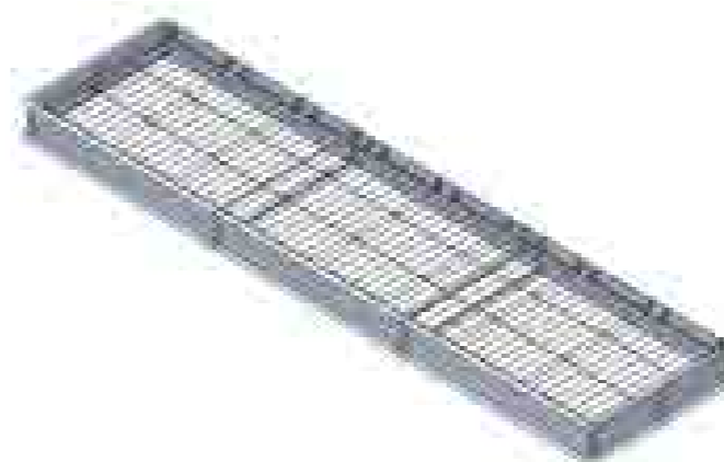
Fig.129 Safety net installed in continuous rooflight
