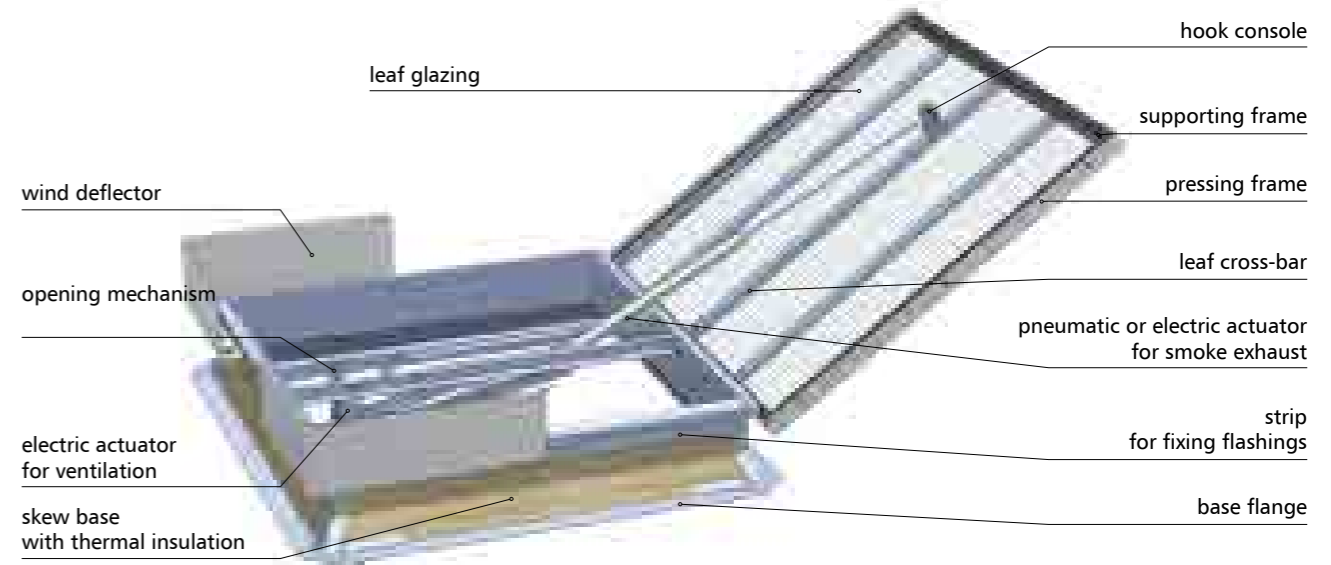
Fig.7 Design of mcr PROLIGHT NG-A smoke vent equipped with wind deflectors, with pneumatic actuator for smoke exhaust and electric actuator for ventilation
