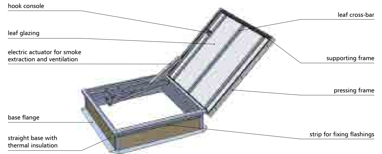
Fig.52 mcr PROLIGHT C100 smoke vent with roof access function and electric control for smoke extraction and ventilation
